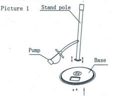
3. Connection for waterway and circuit Put stand pole, fan main body, and connection pole on the ground, connect the hose and celerity tie-in, joint insert parts well, lay in connection pole reasonable, then insert connection pole to sleeve, tighten the M6 bolt. Then put the fan main body into connection pole, tighten screw. Refer to picture 3.
